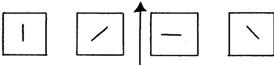
The photometer will measure light attenuation of the spacecraft window due to scattering. While the spacecraft is oriented the astronauts will view a pattern of panels laid out near Laredo, Texas and record their findings. Viewings will be correlated with laboratory experiments and vision will be checked pre- and post-flight.
